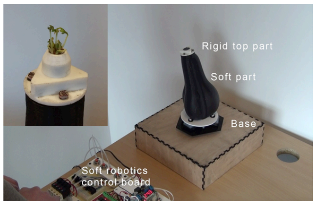
Figure 10. Phytomatic 01 (2016). The robotic part of the system and the rigid tip of the robot with the three LDRs and cress plants. © Jonas Jørgensen
