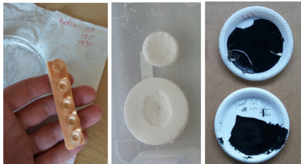
Figure 6. Examples of material experiments. Left: Coloured EcoFlex silicone and beads of hydrogel were submerged in water. The beads become transparent, swell and expand the silicone. Middle: Silicone embedded with kitchen salt then cured in an oven and placed in water overnight to dissolve the salt. The resulting structures were easily compressible and sponge-like with perforated holes all the way through which allows air to pass from one side to the other. Right: Cured sheets of silicone doped with carbon black to yield electrical conductivity (the attempt was unsuccessful). © Jonas Jørgensen
